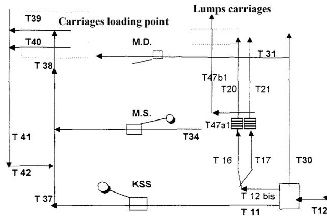
Fig. 2. Diagram of the technological flow at the Corbu coal storage facility
